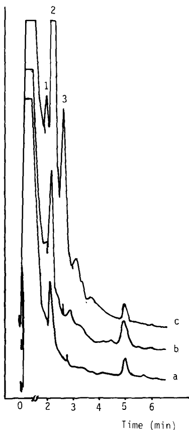
Fig. 3. Chromatograms of (a) derivatized extract of drug-free plasma; (b) underivatized extract of spiked plasma; (c) derivatized extract of spiked plasma containing 600 ng/ml diclofensine. Peaks: internal standard, imipramine (1), endogeneous (2), diclofensine (3).
